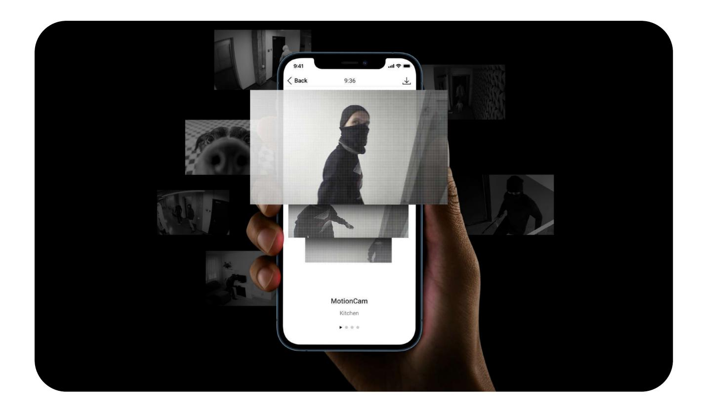
The detector is equipped with a built-in camera and provides the security company and users with animated photos. It features three types of photo verification: by alarm, by scenario, and on demand. Photo verification helps assess the situation at the protected facility, check whether the alarm is real, and respond accordingly.
